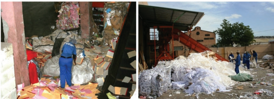
Figure 3. Worker at buy-back centre busy sorting the paper, and paper fed into a baling machine. Photos: David Viljoen.
