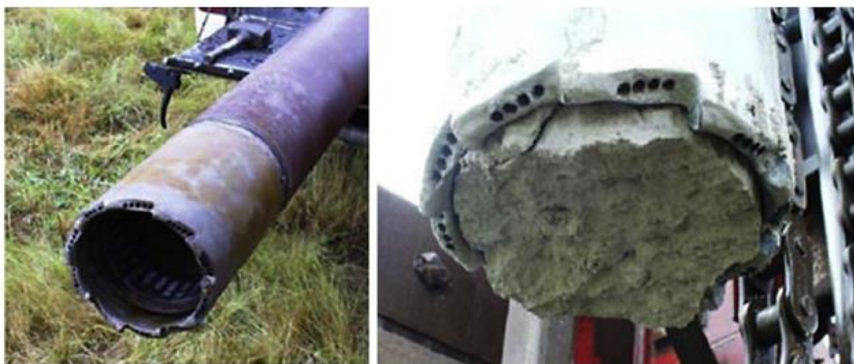
Fig. 1. Air flush core barrel and core inside the barrel.
