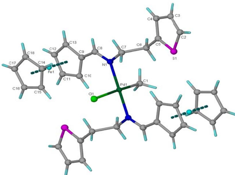
**Fig. 2** X-ray crystal structure of complex **6**
