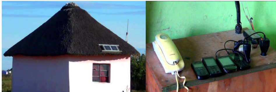
Figure 1: Solar panel and mesh router unit (left) and charging station for mobile phones (right)
