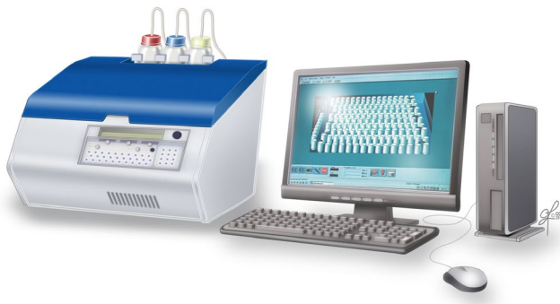
FIGURE 3 Autumat 953 Plus Luminometer used in the measurement of reactive oxygen species (ROS) by chemiluminescence assay. Multiple tubes can be loaded simultaneously for measuring ROS. The luminometer can be connected with a computer and monitor
