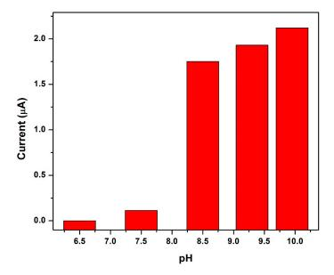
**Figure 14.** Dependence of electrolyte pH on the stripping peak currents of  $Ni^{2+}$  at the NGr-DMG-GCEs in  $0.1 \, M \, NH_3/NH_4Cl$  buffer as electrolyte solution.
