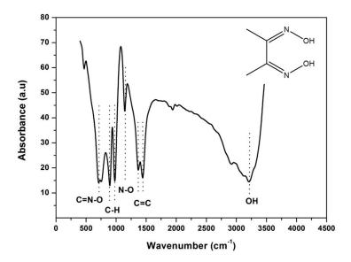
**Figure 1.** Fourier transform infrared spectrometry of dimethylglyoxime as a KBr pellet. Inset: schematic representation of the dimethylglyoxime structure.
