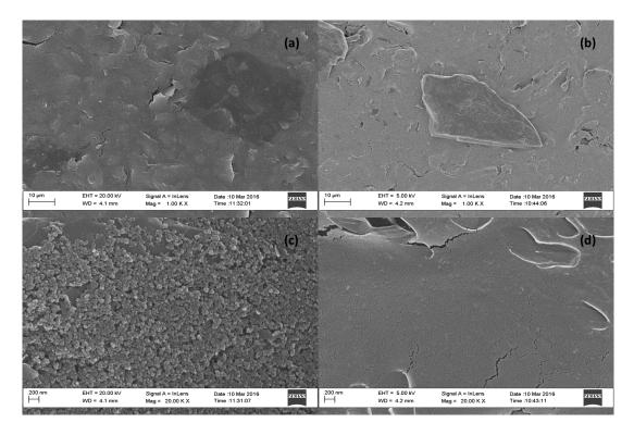
**Figure 4.** High resolution scanning electron microscope (HRSEM) image of ( $\mathbf{a}$ , $\mathbf{c}$ ) Bare SPCE and ( $\mathbf{b}$ , $\mathbf{d}$ ) NGr-DMG-SPCE at  $1000 \times$  and  $20,000 \times$  magnification.
