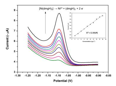
Figure 17. SWAdSV and corresponding calibration plot of the individual analysis of Ni<sup>2+</sup> in the presence of Co<sup>2+</sup> and Zn<sup>2+</sup> obtained at a NGr-DMG-GCE over 2–20  $\mu$ g L<sup>-1</sup>. Supporting electrolyte (0.1 M NH<sub>3</sub>/NH<sub>4</sub>Cl Buffer (pH 9.3)), deposition potential (–0.7 V), deposition time (120 s), frequency (20 Hz), amplitude (0.02 V) and voltage step (0.005 V).
