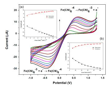
**Figure 6.** Electrochemical characterization of N-DMG-GCE in 5 mM Fe(CN) $_6$ <sup>3-/4-</sup> at scan rate of 10–100 mV s<sup>-1</sup> in supporting electrolyte (1 M KCl). Insets: plots of peak currents vs. (**a**) scan rate1/2 and (**b**) scan rate of the main oxidation and reduction waves.
