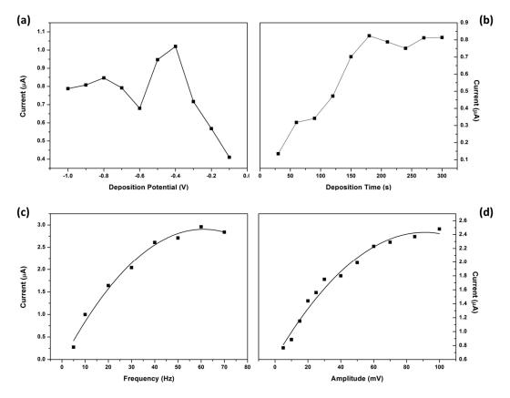
Figure 13. Effect of instrumental parameters; (a) deposition potential; (b) deposition time; (c) frequency and (d) amplitude on the stripping peak current of 10  $\mu$ g L<sup>-1</sup> Ni<sup>2+</sup> at NGr-DMG-GCE. Supporting electrolyte (0.1 M NH<sub>3</sub>/NH<sub>4</sub>Cl Buffer (pH 9.3)).
