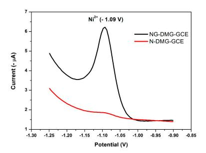
Figure 11. SW-AdCSV of 20  $\mu$ g L<sup>-1</sup> Ni<sup>2+</sup> at N-DMG-GCE (red) and NGr-DMG-GCE (black) with a characteristic reduction stripping potential of -1.09 V. Supporting electrolyte (0.1 M NH<sub>3</sub>/NH<sub>4</sub>Cl Buffer (pH 9.3)), deposition potential (-0.7 V), deposition time (120 s), frequency (20 Hz), amplitude (0.02 V) and voltage step (0.005 V).
