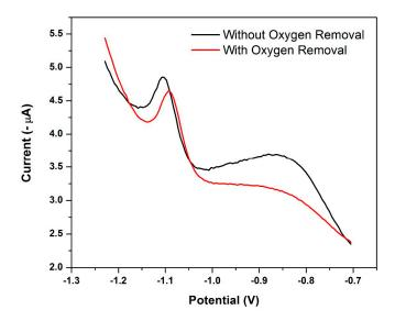
Figure 15. Square-Wave Voltammogram of 4  $\mu$ g L<sup>-1</sup> Ni<sup>2+</sup> at a NGr-DMG-GCE before deoxygenation (black) and after deoxygenation (red). Supporting electrolyte (0.1 M NH<sub>3</sub>/NH<sub>4</sub>Cl Buffer (pH 9.3)), deposition potential (-0.7 V), deposition time (120 s), frequency (20 Hz), amplitude (0.02 V) and voltage step (0.005 V).
