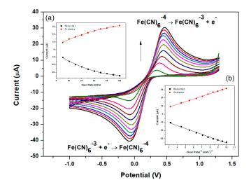
**Figure 7.** Electrochemical characterization of NGr-DMG-GCE in 5 mM Fe(CN) $_6$ <sup>3-/4-</sup> at scan rate of 10–100 mV s<sup>-1</sup> in supporting electrolyte (1 M KCl). Insets: plots of peak currents vs. (**a**) scan rate and (**b**) scan rate1/2 of the main oxidation and reduction waves.
