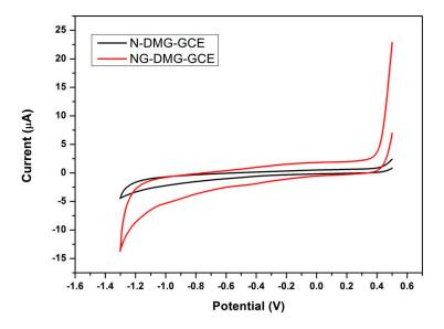
**Figure 10.** Cyclic voltammograms of N-DMG-GCE (black) and NGr-DMG-GCE (red). Supporting electrolyte 0.1 M NH $_3$ /NH $_4$ Cl Buffer (pH 9.3), scan rate (10 mV s $^{-1}$ ), deposition time (120 s), frequency (20 Hz), amplitude (0.02 V) and voltage step (0.005 V).
