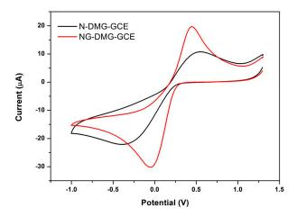
**Figure 8.** Cyclic voltammograms of 5 mM Fe(CN) $_6^{3-/4-}$  at N-DMG-GCE (black) and NGr-DMG-GCE (red) in supporting electrolyte of 1 M KCl at scan rate 50 mV s<sup>-1</sup>.
