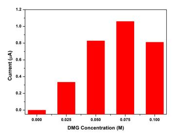
**Figure 12.** Influence of dimethylglyoxime concentration (0–0.1 M) on the stripping peak currents of Ni<sup>2+</sup> at the NGr-DMG-GCEs in 0.1 M NH<sub>3</sub>/NH<sub>4</sub>Cl buffer (pH 9.3).
