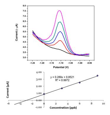
**Figure 18.** SWAdSV and corresponding standard addition calibration plot of the individual analysis of  $\rm Ni^{2+}$  in the presence of  $\rm Co^{2+}$  and  $\rm Zn^{2+}$  obtained at a NGr-DMG-GCE in real tap water samples. Supporting electrolyte (0.1 M NH<sub>3</sub>/NH<sub>4</sub>Cl buffer (pH 9.3)), deposition potential (-0.7 V), deposition time (120 s), frequency (20 Hz), amplitude (0.02 V) and voltage step (0.005 V).
