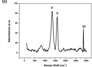
**Figure 3.** Selected structural and morphological characterization of synthesized graphene: (a) high resolution transmission electron microscopy (HRTEM); (b) high resolution scanning electron microscopy (HRSEM) and (c) raman spectroscopy.
