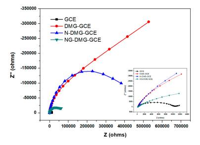
**Figure 9.** Nyquist plots at GCE (black); DMG-GCE (red); N-DMG-GCE (blue) and NGr-DMG-GCE (green) in 5 mM Fe(CN) $_6$ <sup>3-/4-</sup> containing 1 M KCl. Inset is the magnified Nyquist plot between 0 and 12 k $\Omega$ . The frequency range is between 0.1 and 100,000 Hz.
