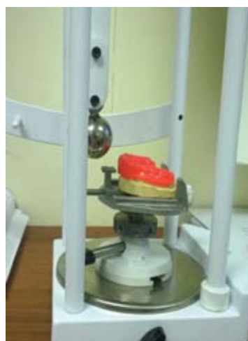
Figure 1: Pendulum type impact testing machine.
