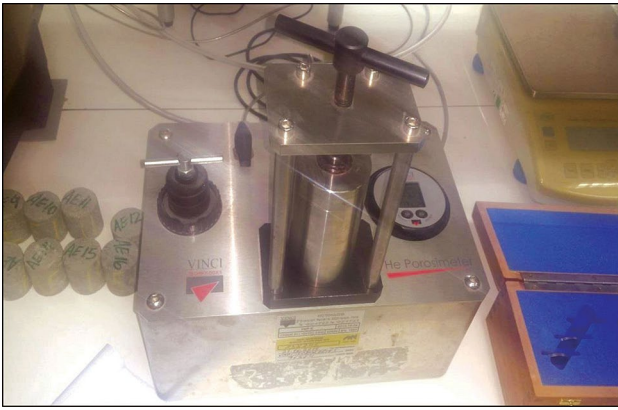
Fig. 3 Porosimeter instrument used to measure the porosity of the core plugs
