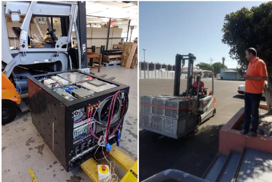
Fig. 4 – Left – shows 15 kW – PEMFC power module before installation in STILL RX60-30 forklift. Right – Prof. I. Tolj (FESB, Split) supervises VDI-60 test of the forklift (Cape Town, South Africa).
