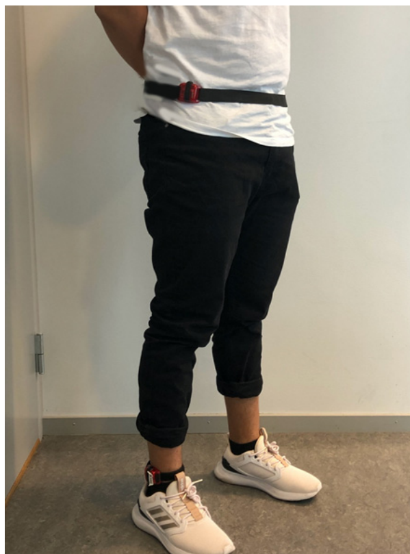
Figure 1. ActiGraph positioned around the right waist (above the iliac crest) and right ankle (proximal to the lateral malleolus).
