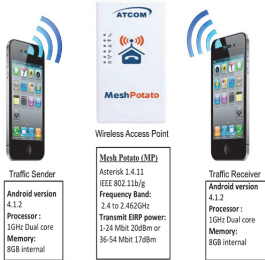
Figure 3: Wireless testbed network setup.
