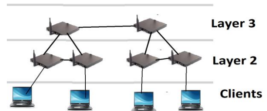
Figure 5: The new wireless mesh architecture
