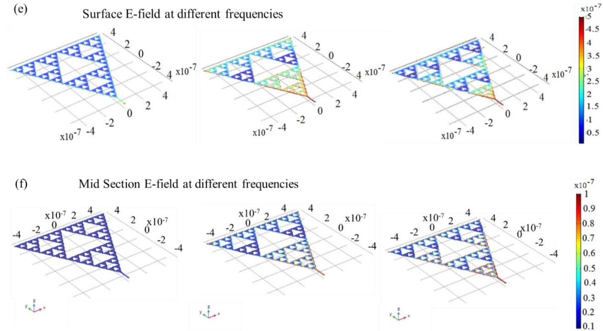
**Figure 2.** (a) Sierpinski antenna model. (b) Sierpinski Global S-parameter (in dB) vs. frequency with three resonances at 35, 110 and 215 THz. (c) Sierpinski far-field polar coordinate patterns at selected frequencies. (d) 3D emission patterns. (e) Sierpinski surface E-fields at the resonance frequencies. (f) Sierpinski mid-section E-fields at the resonance frequencies.
