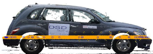
FIGURE 10. LiDAR scanned structure. This figure illustrates image artifacting caused by a reflective surface image obtained from D.S. Dima et al. [241].
