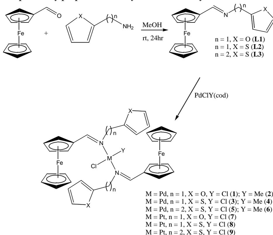
**Scheme 1:** Preparation of *trans*-bis(ferrocenylimine) Pd(II) and Pt(II) complexes **1** – **9**
