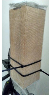
Figure 3: Hand built Faraday cage for shielding MPAWD
