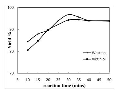
**Figure 4.** Effect of reaction time on FAME yield via the mechanical stirring under a 6:1 methanol/oil ratio, at  $60 \degree C$  and catalyst concentration of 1% wt of oil.
