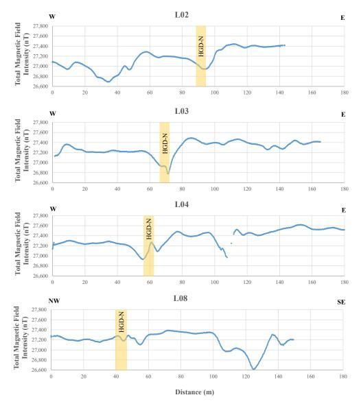
Figure 5. Profile plots of the total magnetic field recorded along the lines L02, L03, L04, and L08.
