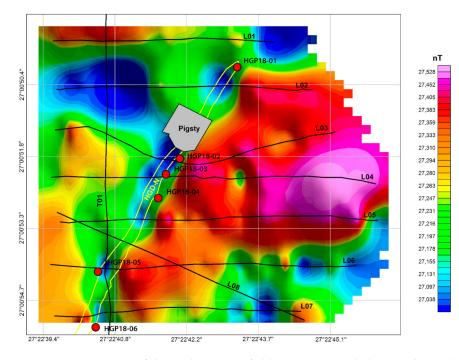
**Figure 6.** Contour map of the total magnetic field intensity recorded across the northern outcrop of the Holfontein Granophyre Dike (HGD-N). Data collection lines are indicated in black. Geological samples are indicated with red points.
