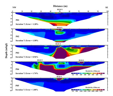
**Figure 7.** Modeled resistivity sections across the HGD-N and HGD-S outcrops. The legend for profiles P01–P04 is located in profile P04. Due to the much higher resistivities recorded along profile P05, a different color scale is used for the resistivity model of this profile. mgbl: meters below ground level.
