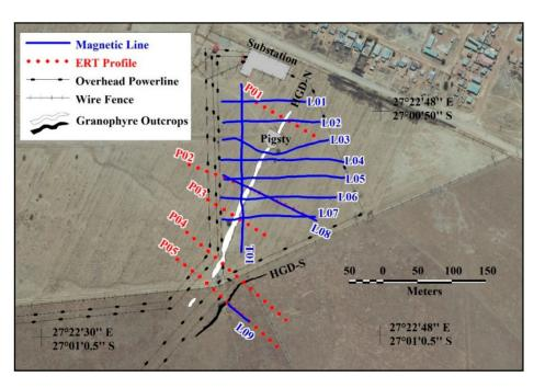
**Figure 3.** Positions and orientations of the magnetic lines and electrical resistivity tomography (ERT) profiles across the Holfontein Granophyre Dike (black lines) plotted on top of an aerial photo.
