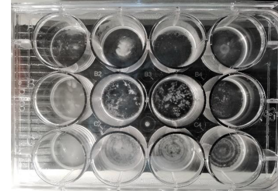
Figure 2. Forty-eight hour bulk biofilm formation seen at the bottom of 12-well cell culture plates, after cells were washed and before CFW/KOH staining and FM observation.
