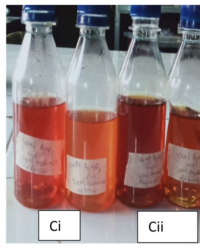
Mixture of extract and silver nitrate (Ci – aqueous extract-mediated; Cii- ethanol extract-mediated)
